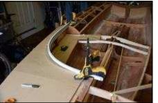
Cardboard templates are made for the deck panels, these are then cut out from two sheets of Tiger striped sapele along with the seat tank tops
