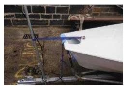
Bow tied to stop boat sliding back when being towed
